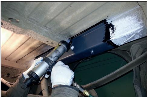
10. Spray the area, where the protective coating was removed, with an anti-corrosive protection
