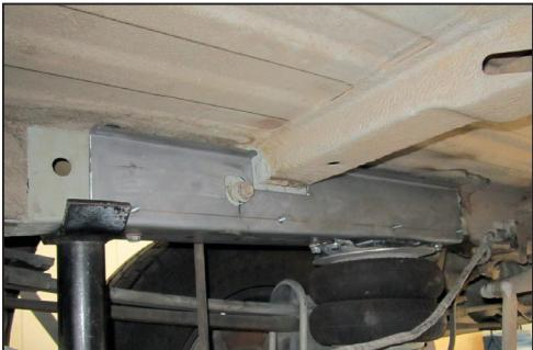
9. Seal all edges of the chassis reinforcement bracket, so moisture and dirt can't get between the chassis and bracket. Use the glue to seal the edges.
