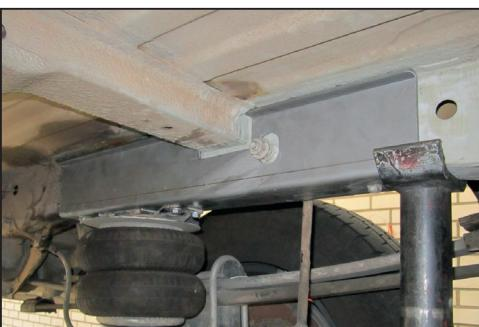
7. Mount the air spring assembly to the chassis reinforcement bracket.
