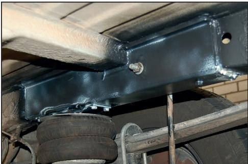
11. Press the fixing ties on the weld studs. Fasten the wiring harness to the chassis reinforcement bracket using the fixing ties.
