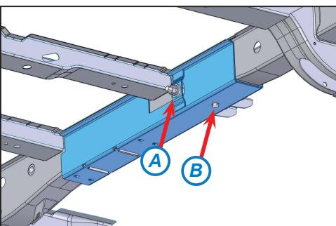
\*\* If the vehicle isn't equipped with a roll stabiliser, use these bolts, nuts and washers. Always use washer M12 Ø30 on the inside of the chassis.
