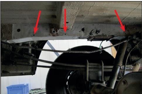
3. Apply some glue to the chassis, in the area where the (bump stop bracket) plate will be placed.
