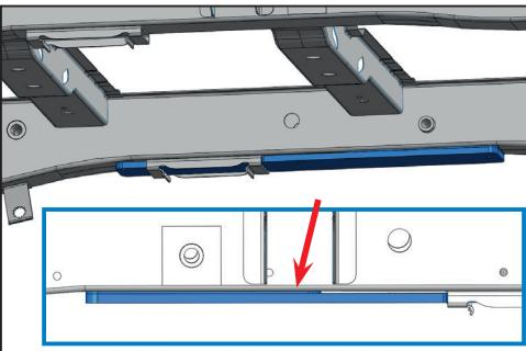
5. Apply some glue to the inside of the chassis reinforcement bracket.
