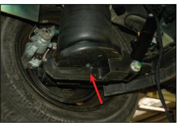
Connect the air tubes to the air springs. Loosen the end of the air connector and slide this over a piece of air tube.
