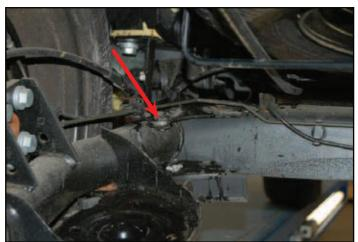
5. Remove the rivet on the marked place. Remove it on both sides of the vehicle!
