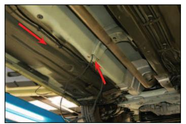
5. Lead the wire across the sub frame, along the steering house, to the chassis. From there lead the wiring along the chassis to the front of the vehicle.
