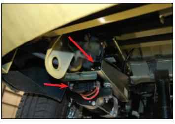
Now lead the air tubes to the valve block and cut it to the right length. Connect the air tube to the correct position on the valve block.
