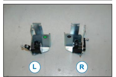
5. Fit the heightsensors on the outside of the chassis. To fit this, use the original bolts on the same holes as the original shock absorber was mounted. Use the special washers *between* the chassis and the support!
