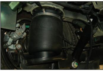
5. Use the tapping screws and washers to secure the bottom of the air spring to the rear axle.
